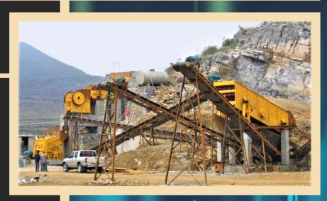
START CRUSHING AND SCREENING VARIOUS MATERIALS, UP TO 700 TON PER HOUR.
