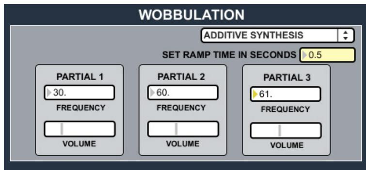
The wobbulation section is meant to be interfaced with a DIY electromagnet through an audio amplifier, using Kyle Evans' tutorial on hacking a cathode ray tube with a DIY electromagnet at crackedraytube.com. Kyle's instrumentation is a based on the Paik-Abe synthesizer, also known as the wobbulator.
