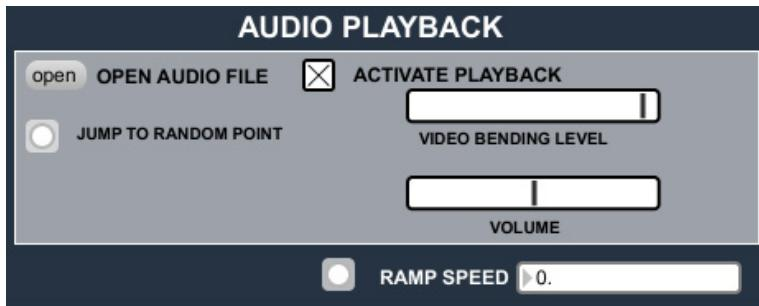
The audio playback section enables an audio file to be bent into video via outputs 1 and 2 (and the VGA cable modified to bend audio into video). It also enables the same audio file to be sent to the speakers via outputs 3 and 4.
