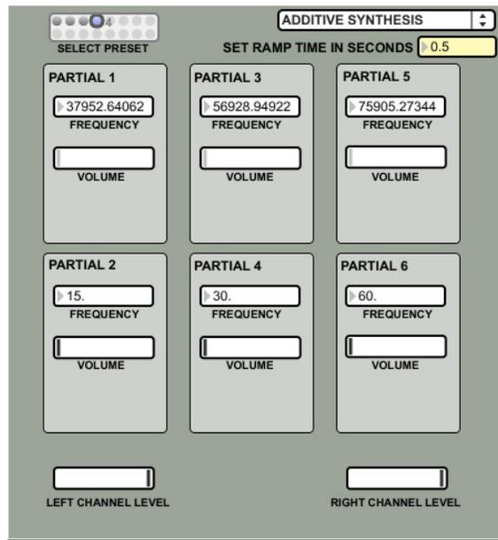
The first mode of sine wave synthesis is Additive Synthesis: synthesis of multiple basic waveforms (6 if using one signal, or 12 if using both signals). Additive synthesis generates a *composite* tone through multiple *partials*,
