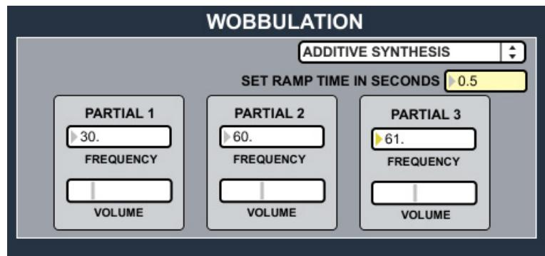
The wobulation section is meant to be interfaced with a DIY electromagnet through an audio amplifier, using Kyle Evans’ tutorial on hacking a cathode ray tube with a DIY electromagnet at crackeddraytube.com. Kyle’s instrumentation is based on the Paik-Abe synthesizer, also known as the wobulator.
