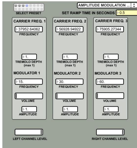
The second mode of sine wave synthesis is Amplitude Modulation: varying the amplitude (or strength) of a *carrier* frequency with a *modulating* frequency that is altered by a *tremolo depth*.
