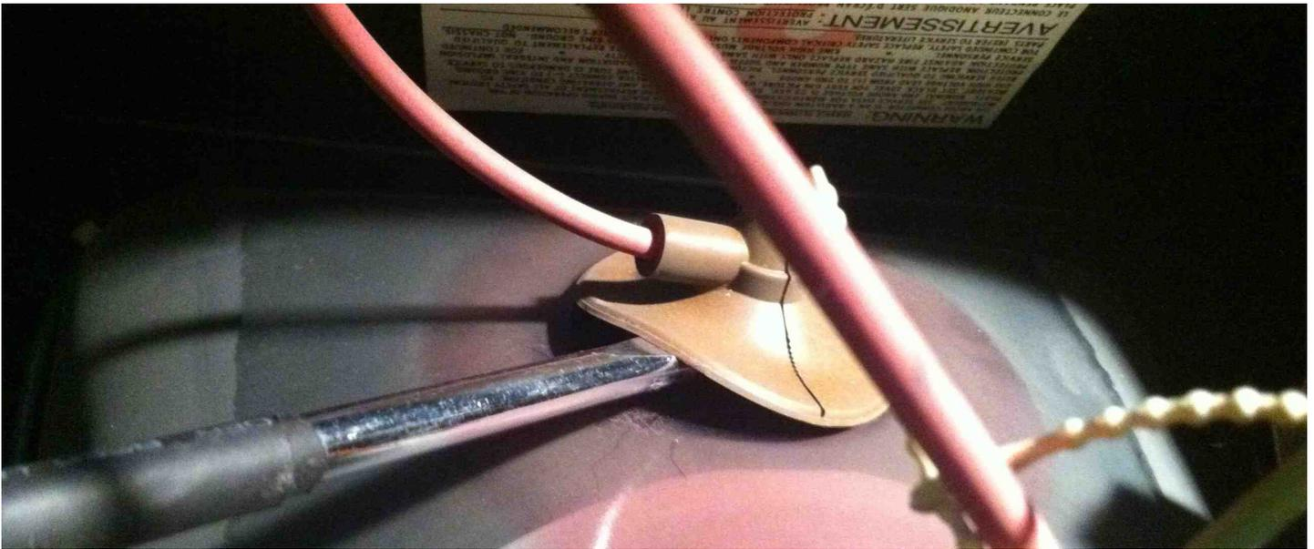
At this point, leave the screwdriver in place for a couple minutes to ensure that all the electricity has been discharged. After that, try discharging it one more time just to be safe. Now you have a safely discharged TV to work with.
