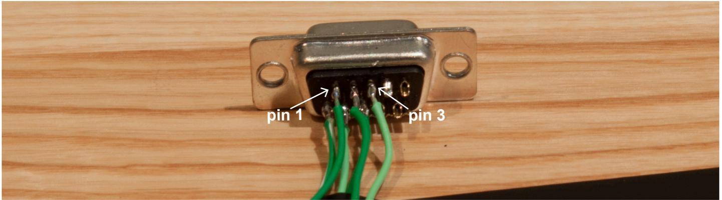
3. Apply heat shrink tubing at this point if you're using it.
