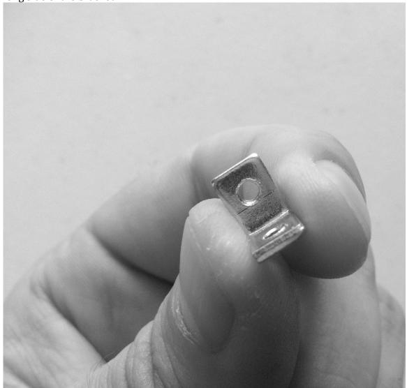
The L-Bracket is secured to the spacer using a 4-40 screw. Once the mounts have been assembled, they should be screwed into the front panel first. The SD Card PCB should be secured to the mount only after all other boards have been assembled, at the very end of the build.
