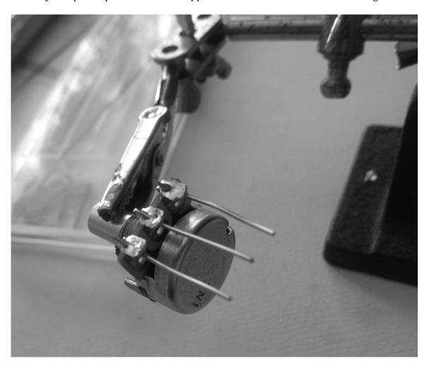
A fully prepared pot. Bus bar has been clipped close to the lugs, and the anti-rotation tab has been removed:
