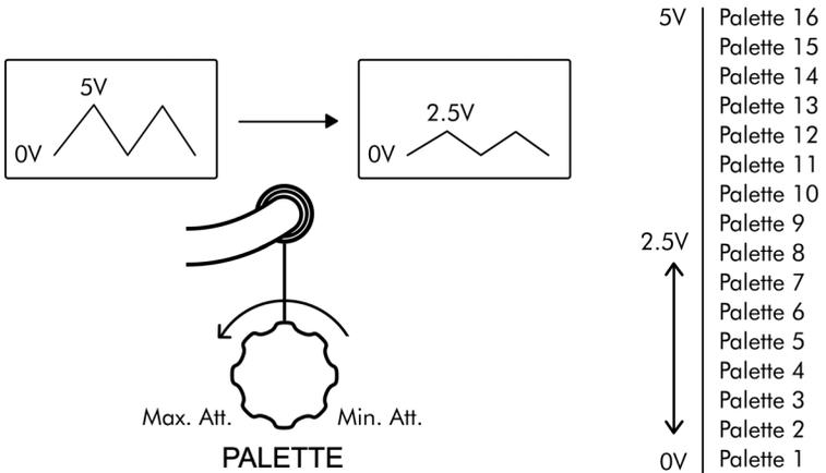
By adjusting the amount of attenuation, it's possible to format higher voltage signals to match the WORLD CORE's 0-5V responsive range, or to truncate the number of selectable states as shown above. Note that attenuation only affects the top end of the voltage
