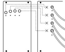
No functionality is lost when using **NORMALIZATION**. The **DIRECTIONAL OUTPUTS** can still be routed to other locations as usual, and the internal connections can be overridden by simply inserting a patch cord into the corresponding **DIRECTIONAL INPUT**.
