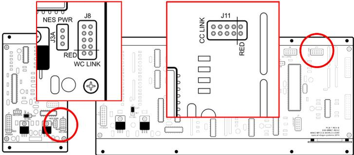
Position the cable's **RED STRIPE** so that it aligns with the pins marked **RED** on the **WC LINK** and **CC LINK** header connectors. Due to its position on the **MOTHERBOARD**, you will have to rotate the cable 90 degrees to the left when connecting it to the **CC LINK** header on the **WORLD CORE**.
