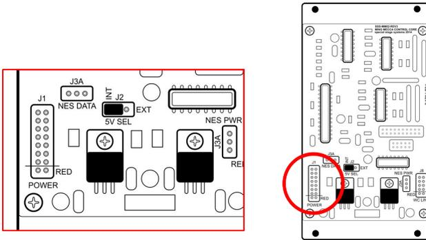
The 16-to-16 pin POWER CABLE should already be connected to the module. Note the position of the cable's RED STRIPE. Verify that the RED STRIPE is aligned with the location marked "RED" on the power connector. If the cable is not properly aligned, remove and reposition it so that the alignment is correct.
