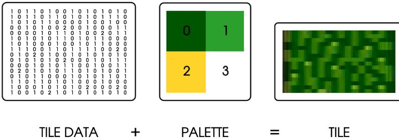
The **WORLD CORE** can store a total of 32 **TILE DATA** bitmaps and 16 **PALETTEs**, which are loaded either from a user-created bank (if a **WORLD PACK** is loaded into the **CARTRIDGE SLOT**) or from the default internal memory. Although the complete contents of the **TILE** and **PALETTE** data banks are always accessible, the **WORLD CORE** can only render two **TILEs** onscreen at any given time.
