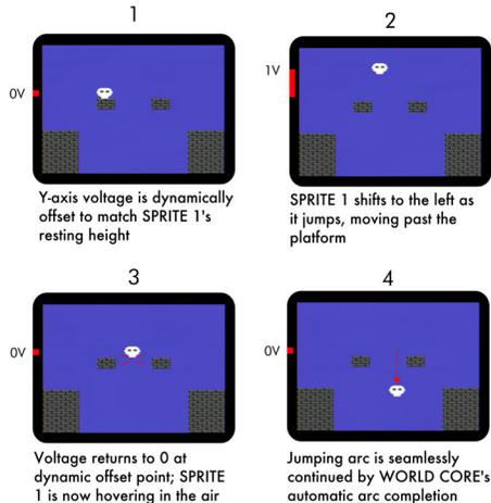
ramp to complete the arc instead. This arc is generated by analyzing the incoming **Y CV** input voltage and computing its speed in realtime, so that no matter the speed of the incoming arc, the **WORLD CORE** will complete it seamlessly.
