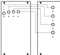
The directional outputs can still be patched to other locations without breaking the internal connections
