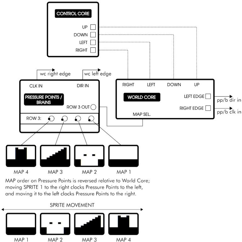
As **SPRITE 1** moves across the wrap boundary, it causes two closely spaced **EDGE COLLISION** events. If **SPRITE 1** is moving to the right, for example, it will cause the **RIGHT EDGE** output to fire as it approaches the edge of the screen, immediately followed by the **LEFT EDGE** output when it reappears on the opposite side. The same effect occurs if the **SPRITE** is moving to the left, except that the order of the **EDGE COLLISION** events is reversed.
