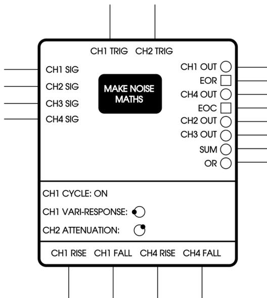
MATHS has signal, TRIGGER, and CV inputs, as well as a variety of outputs, so all four sides of the box are used. Various module states are noted in the parameters box, including the position of the cycle toggle on Channel 1. GATE outputs like end-of-rise (EOR) and end-of-cycle (EOC) are accompanied by a square symbol. The full legend of possible output symbols is shown to the right.
