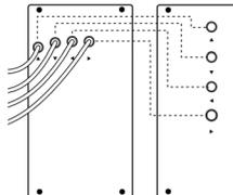
Normals break when patch cords are inserted into the directional inputs.
