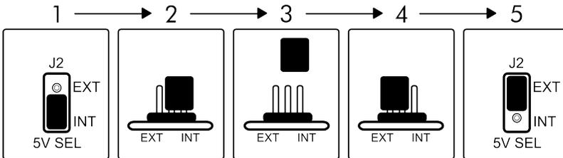
**WARNING:** the 5V SELECT JUMPER must be installed in either the “EXT” or “INT” position before applying power. **Never attempt to power the WORLD CORE with the 5V SELECT JUMPER removed.**
