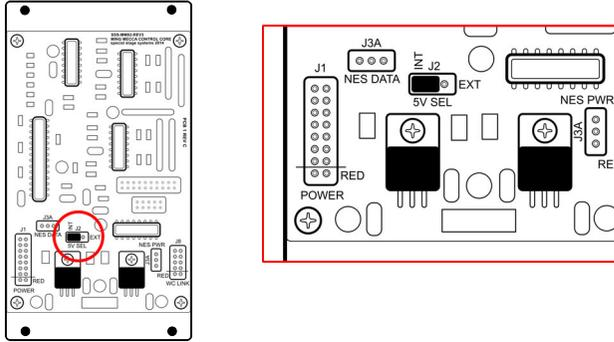
Remove the jumper and reinstall it in the "EXT" position, as shown in the diagram below.
