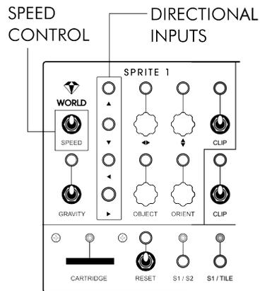
patching a **GATE** signal into one or more of the **DIRECTIONAL INPUTS** will automatically engage relative control for the appropriate direction. Exiting the system is similarly straightforward: to regain absolute X/Y control of **SPRITE 1**, simply patch a voltage into its X or Y CV input (or wiggle its corresponding knob).
