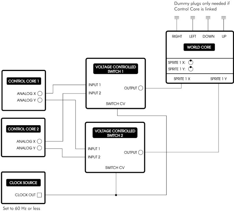
Note that the voltage sources do not have to be CONTROL CORES; any sources can be used, including LFOs, random voltage generators, cycling ENVELOPES, or even static DC offsets. However, for patches where the SPRITE locations are stationary, a better solution is to simply use a STEP SEQUENCER clocked at 60 Hz, eliminating the need for VOLTAGE CONTROLLED SWITCHES.
