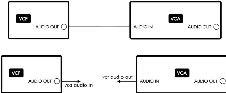
Additionally, only inputs and outputs that are in active use are included within the module boxes. In the following simple patch, the majority of the **WORLD CORE** and **CONTROL CORE I/O** is not shown in the schematic; only the connections relevant to the patch are labeled.
