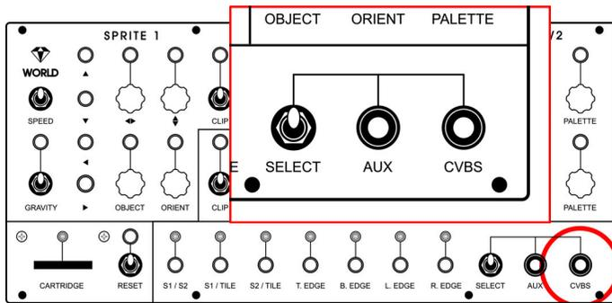
Connect a composite video (RCA) cable to the **CVBS** jack. Make sure you don't accidentally plug into the **AUX** jack instead. Now plug the other end of the cable into your display's video input.
