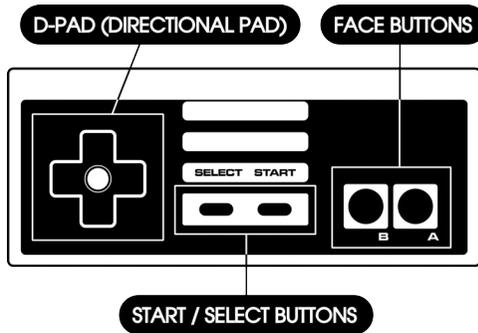
Dedicated **ANALOG X** and **ANALOG Y** outputs provide additional control by converting D-PAD activity into analog CV. This is best understood as a kind of “virtual analog joystick.” Holding **UP** will increase the voltage at the **Y** output, while holding **DOWN** will decrease it; similarly, holding **RIGHT** will increase the voltage at the **X** output, while holding **LEFT** decreases it. The voltage will retain its level even after the button is released.
