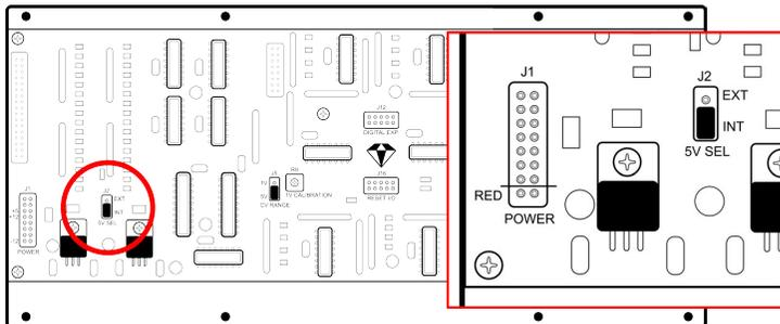
Remove the jumper and reinstall it in the “EXT” position, as shown in the diagram below.
