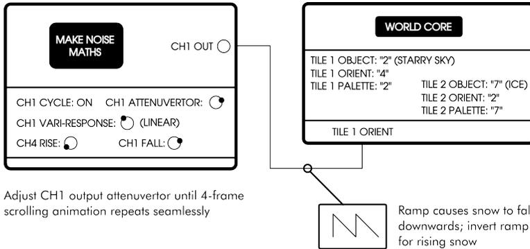
By building the patch above, the four frames indexed by the **ORIENT CV** can be animated in a continuous loop, giving the impression that the snow is falling infinitely. If you don't own a **Make Noise MATHS** you can substitute any standard LFO or cycling **ENVELOPE** generator, so long as it has a 0-5V range and you can control the phase of the ramp (i.e., set a fast attack and slow decay, or vice versa).
