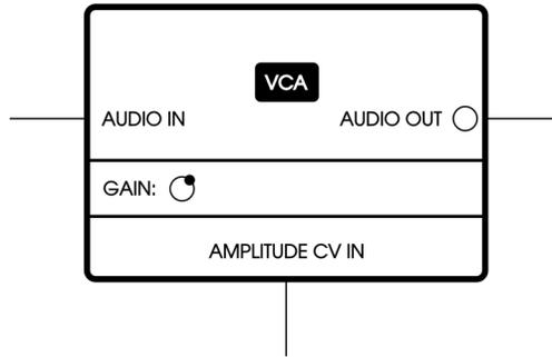
The position of the gain knob is noted graphically in the parameters box, and the inputs and outputs are labeled along the edges. The audio output is accompanied by a circle, which represents a variable or complex waveform. Since this VCA doesn't have any GATE or TRIGGER inputs, the top side of the module is unlabeled and has no connecting lines.
