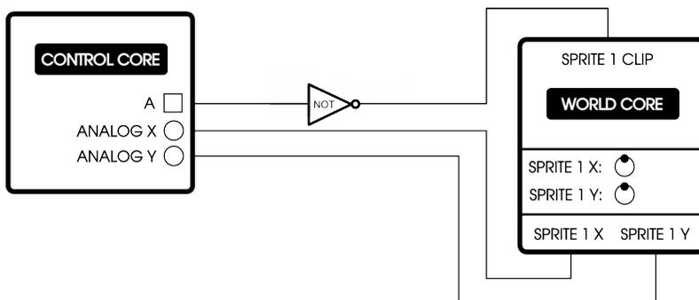
Since the **CONTROL CORE**'s analog **X** and **Y** outputs generate 0-10V signals, the modified patch schematic notes that the **SPRITE 1 X** and **Y** knobs should be at high noon to achieve 50% attenuation, scaling the voltage to the **WORLD CORE**'s 0-5V responsive range.
