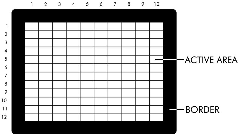
The display consists of an active area with a 160 x 192 pixel resolution, surrounded by an inactive black border. The active area is divided into 120 locations, organized in a 10 x 12 grid. Each grid location is further subdivided into a 16 x 16 pixel bitmap displaying one of two currently selected **TILES**. In order to understand how these **TILES** are selected, rendered, and organized into larger patterns, we will now take a look at how the WORLD CORE processes graphical data.
