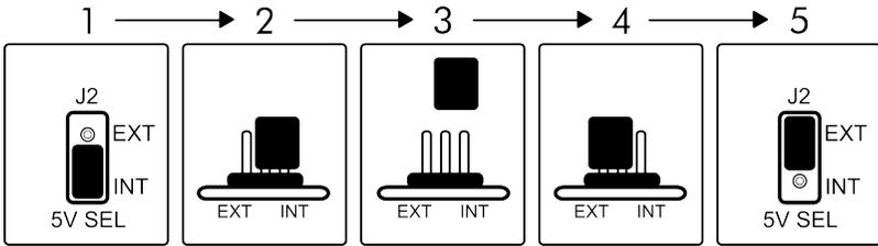
**WARNING:** the 5V SELECT JUMPER must be installed in either the "EXT" or "INT" position before applying power. **Never attempt to power the CONTROL CORE with the 5V SELECT JUMPER removed.**
