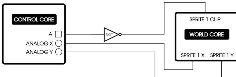
Knobs and toggles at signal destinations are assumed to be fully open unless otherwise noted. In the above patch for instance, the **SPRITE 1 X** and **Y** knobs are fully clockwise (0% attenuation) and the **SPRITE1 CLIP** toggle is in the upward or “ON” position. Non-default positions are simply noted in the parameters box along with the rest of the controls, as shown in the modified version below:
