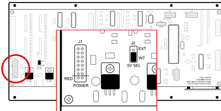
The 16-to-16 pin **POWER CABLE** should already be connected to the module. Note the position of the cable's **RED STRIPE**. Verify that the **RED STRIPE** is aligned with the location marked "**RED**" on the power connector. If the cable is not properly aligned, remove and reposition it so that the alignment is correct.
