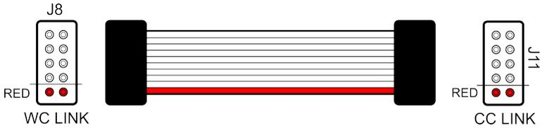
Double-check the **RED STRIPE** alignment, and then firmly press down on each side of the cable connector until the header pins are fully covered. Your **CONTROL CORE** and **WORLD CORE** are now **LINKED**. Only one **CONTROL CORE** can be **LINKED** to a **WORLD CORE** at a time. If you ever decide you would rather keep them functionally isolated, the modules can be **UNLINKED** by removing the cable.
