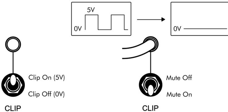
Parameters can also be controlled by patching **GATE** or **TRIGGER** signals into the jack input. Just like knobs, toggles don't directly control parameters when their input is in use. Instead, they become "mute" switches that pass or block the signal patched into the input. The down position turns the mute "**ON**", overriding the signal with **0V**, while the upward position turns the mute "**OFF**", allowing the signal to control the parameter.
