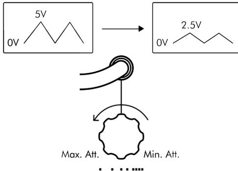
only affects the top end of the voltage range. Additional (third party) modules are required to raise the low end of the range (DC offset summing), or to eliminate negative voltage (rectification).
