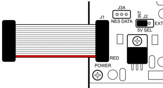
Connect the other end of the cable to your power supply, making sure that the **RED STRIPE** aligns with the **-12V** pins on the **BUSBOARD** header.
