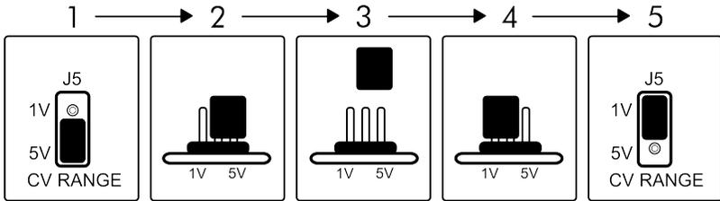
The WORLD CORE will now use a 1V reference for its CV range. Digital GATE and TRIGGER inputs conform to a 0.5V logic threshold by default and require no user configuration for LZx compatibility.
