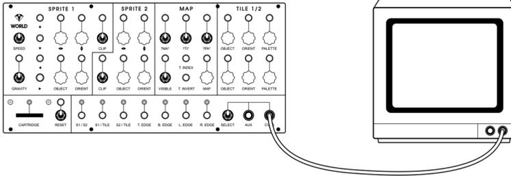
Finally, make sure the **SELECT** toggle is in the upright position. This toggle switch determines whether the CVBS jack will display the **WORLD CORE's** internal video output, or the signal patched into the **AUX** video input. When set in the downward position, it selects the **AUX** input, which will cause the **WORLD CORE** to display a blank screen when nothing is connected to the **AUX** jack.
