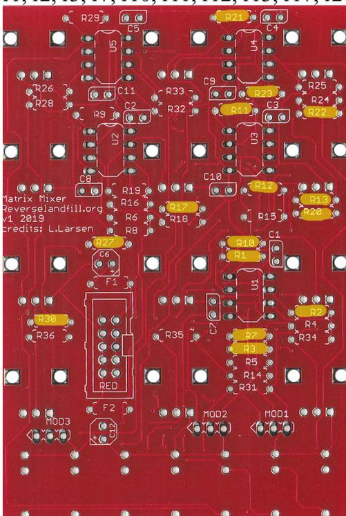
The 6x 3.3k (r4, r14, r24, r34, r35, r36) resistors control the gain of the mixers, the value of 3.3k sets 3x gain.
