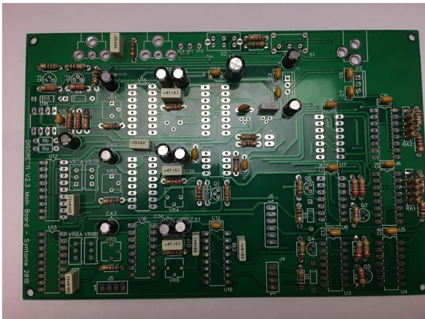
Place all the capacitors according to the bill of material. All the 100nF capacitors are ceramic (yellow body with 104 marking). Mind the orientation of electrolytic capacitors.
