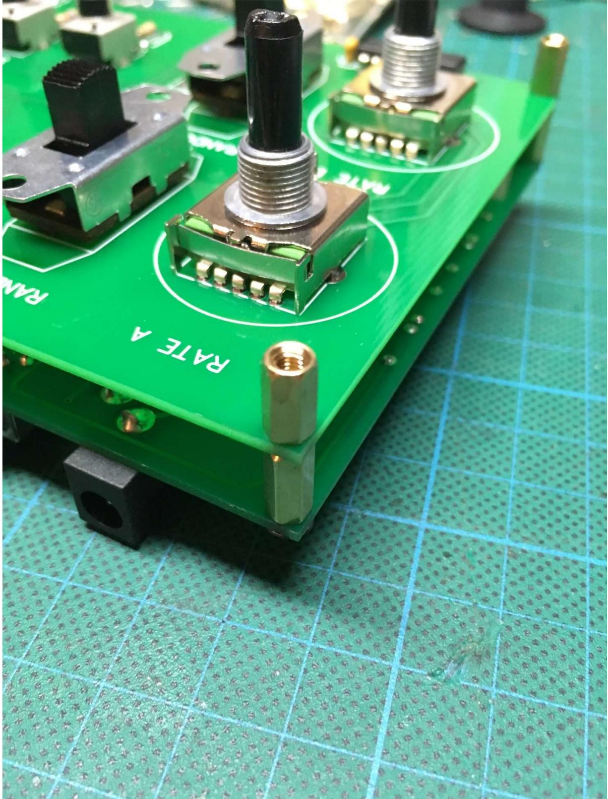
Add the top part of the enclosure, and secure it to the boards using 6mm M3 screws.
