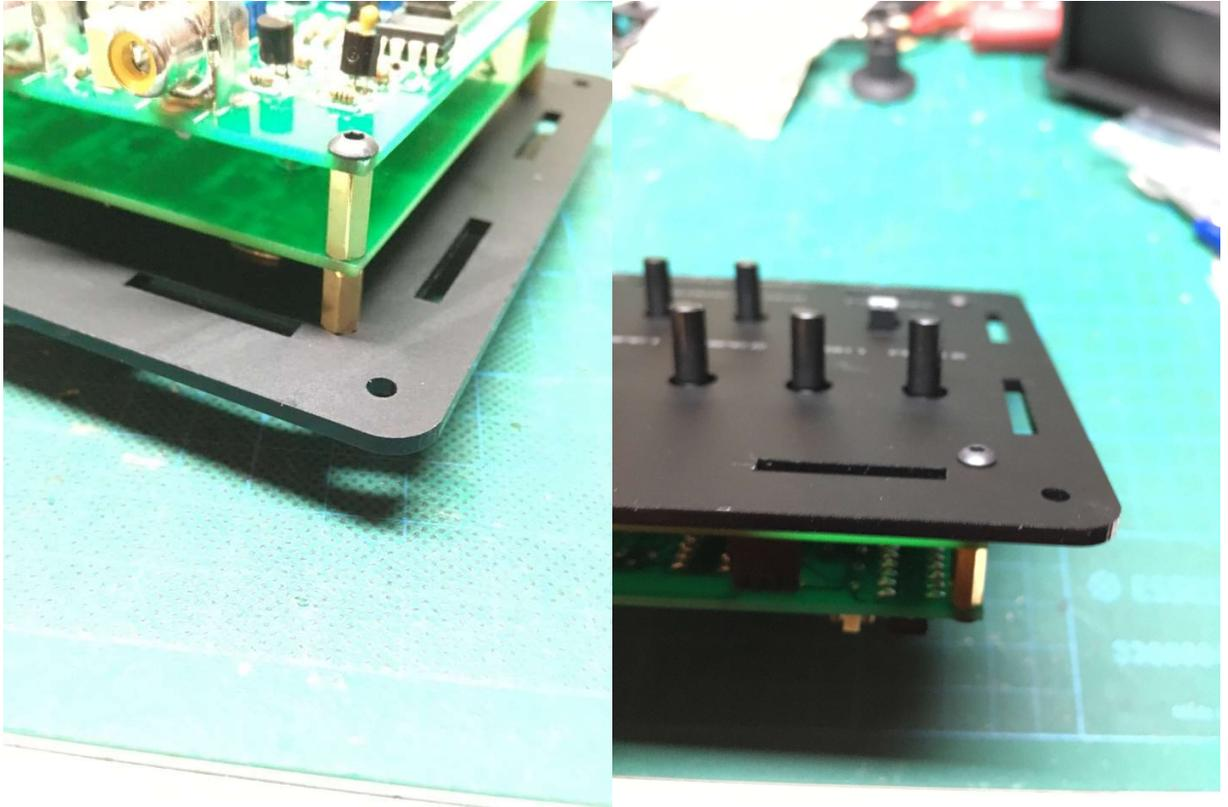
Now, add the two long side of the enclosure, attach the 45mm FF spacers using 6mm M3 screws. Add the 2 short side and the bottom of the enclosure. Attach the rubber feet using 8mm M3 screws.
