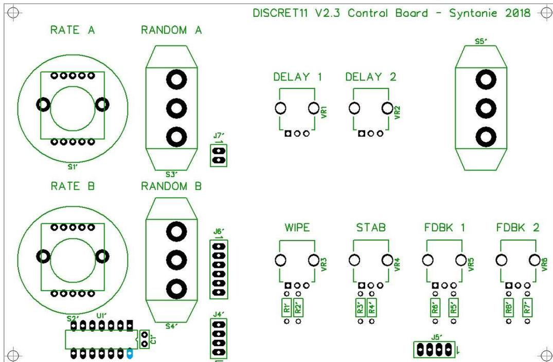
If every voltage measured is correct, you can place all the ICs according to the BOM. Test the voltages at the output of the regulators, if it's still right, you can go to the calibration part. If not, check that every component is at the right spot, with the right orientation. Also check that everything is soldered well and that there is no short.
