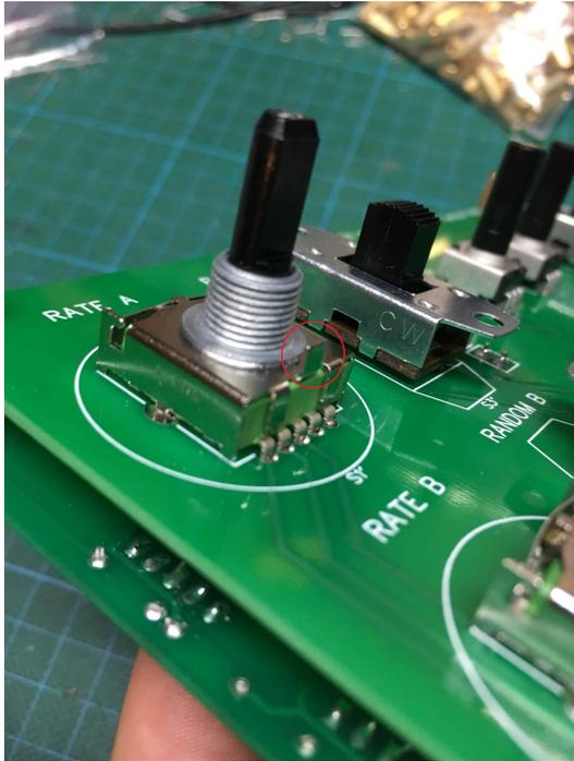
Before soldering the rotary switches, cut the small tabs using cutters, it will be better for the enclosure assembly later.
