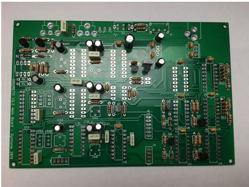
Place all the transistors and diodes according to the bill of material. Mind that Q3 is a 2N3906 whereas all other transistors are 2N3904. Diodes are polarized, be careful to orientation.
