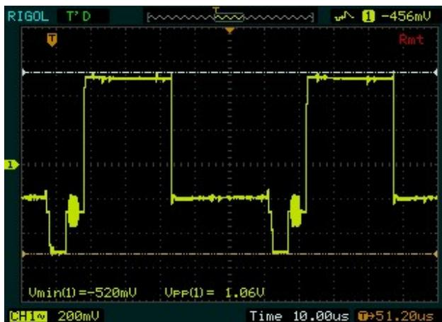
Using VR1, set the amplitude of the signal to 1Vpp (yellow signal on the oscilloscope).
