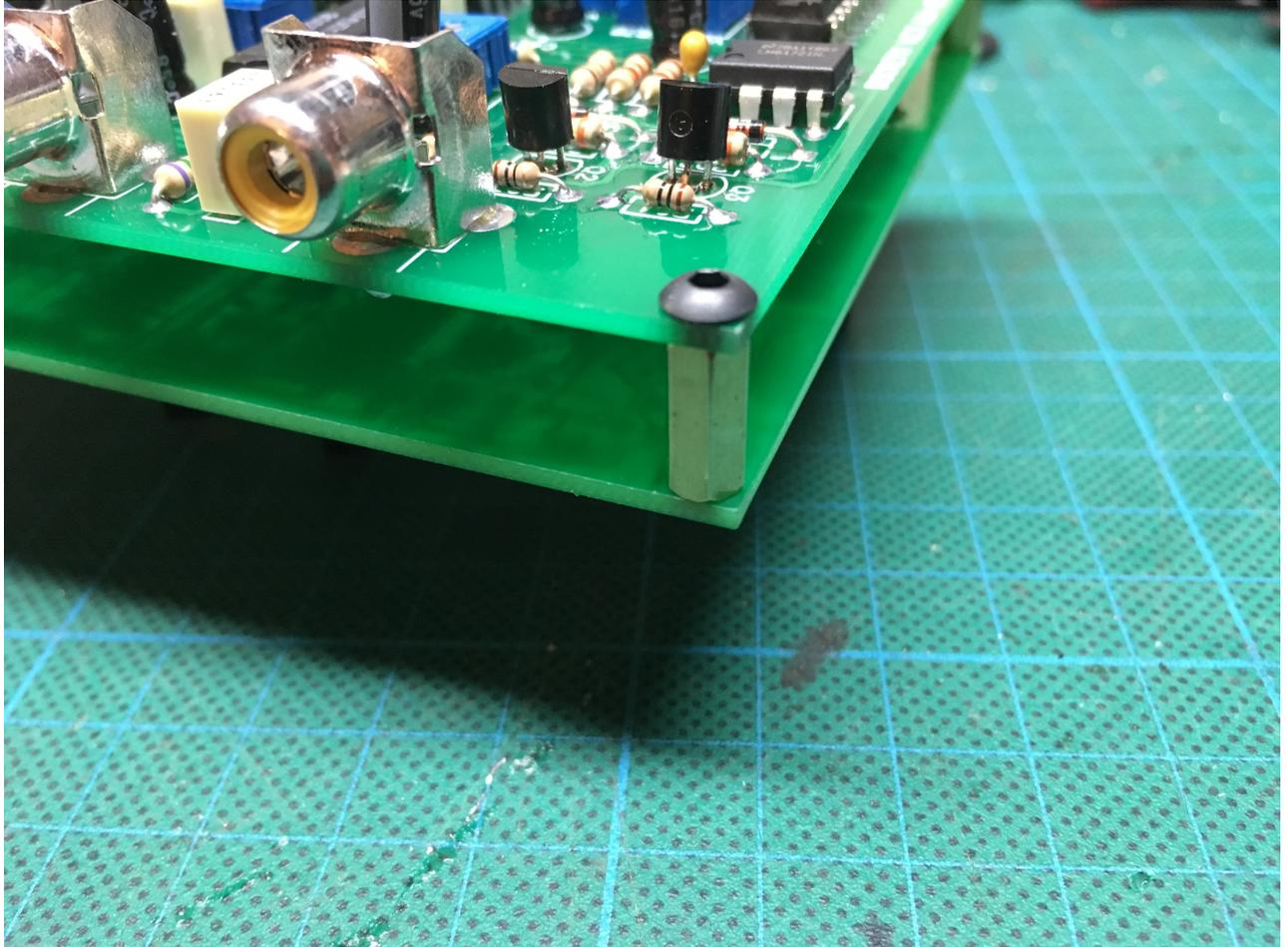
Then add the 9mm spacers (the ones with a thread) on the control board side.
