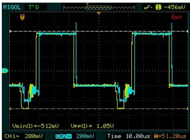
Keep one probe of the oscilloscope on TP1 and put the other one on TP3. Using VR5, set the signal at TP3 so it has the same amplitude as the signal at TP1.
