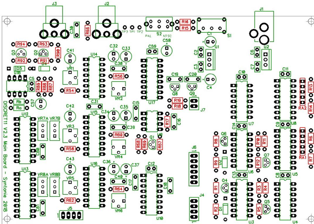
Place all the resistors according to the bill of material.
