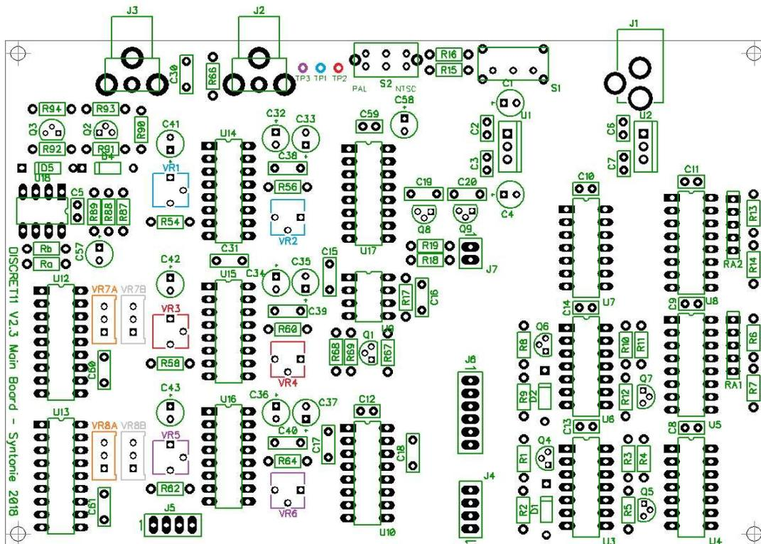
The 3 test points are located between J2 and S2:
