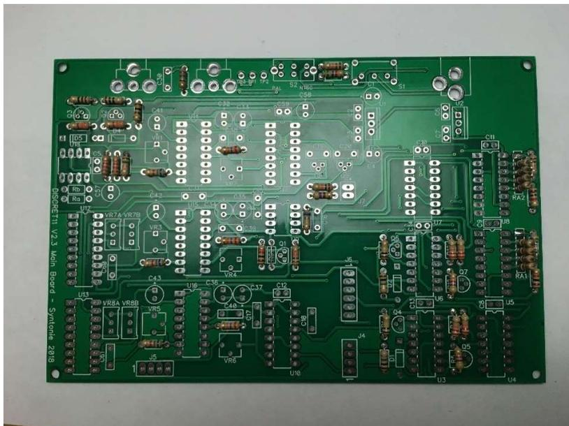
Note that on the picture, RA1 and RA2 are 4x 1K resistor, whereas kit include 2 resistors array (yellow component with 5 legs). Make the dot on the component match the square pad on the component footprint.
