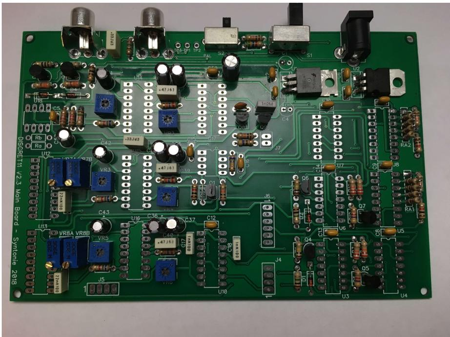
Place both RCA connectors and the DPDT switch. Check the body of the trimmer potentiometer for their value, 502 is 5K, 203 is 20K and 202 is 2K. VR7A and VR8A are used to set delays for NTSC, VR7B and VR8B are used to set delays for PAL. So if you don't intend to use both standards, you do not need to put all 4 trimmers.
