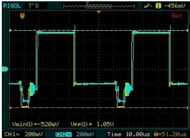
With the other channel of the oscilloscope, check the signal at TP2. Using VR3, set the signal at TP2 (blue trace) so it has the same amplitude as the signal at TP1 (yellow trace), don't worry about the sync signal, it gets deteriorated by the delay but will be replaced by the original sync signal later.
