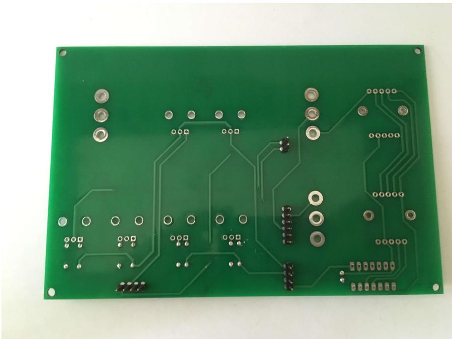
First, place the 4 connectors (J4', J5', J6', J7'). The pins of the connector should be on the solder side of the board.
