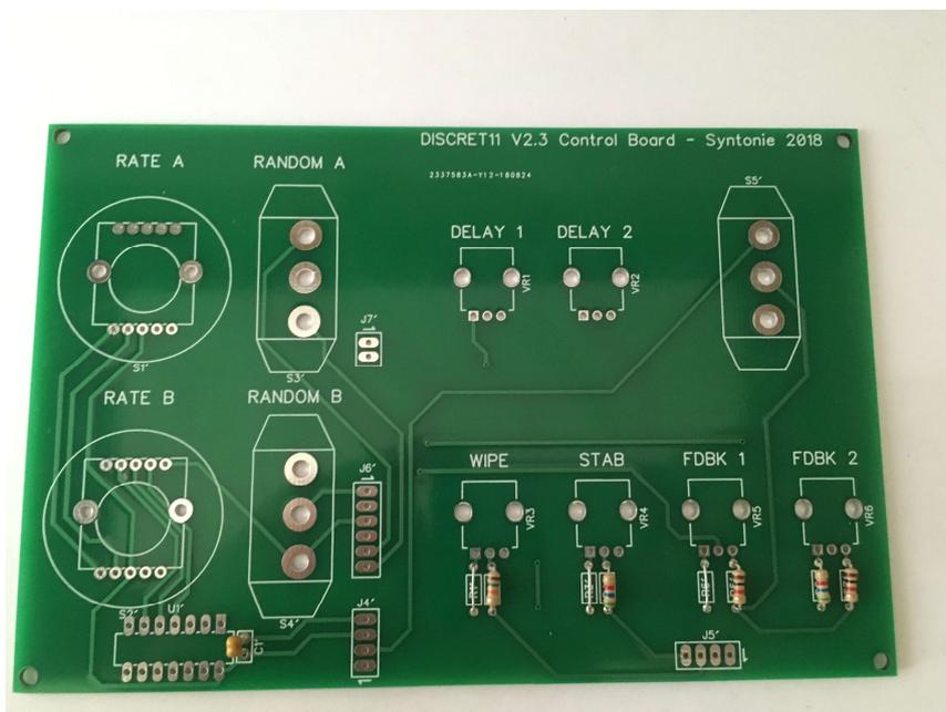
Place the 100nF capacitor (C1'), and all the resistors. Note that R1', R3' and R6' are resistors legs used as jumper.
