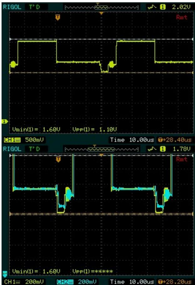
Adjust VR2 until the sync tip is at the right level (here 1.6V).
