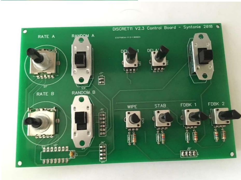
Be careful that all the hardware components sit straight on the board, it will be easier for assembly enclosure later. Now, the control board is almost complete, don't put U1' IC yet, you can however put the IC socket.
