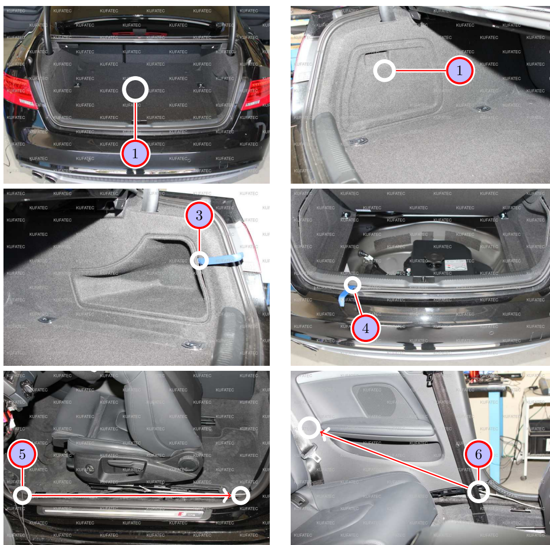
Figure 7: Removing trim panel trunk / cable routing
