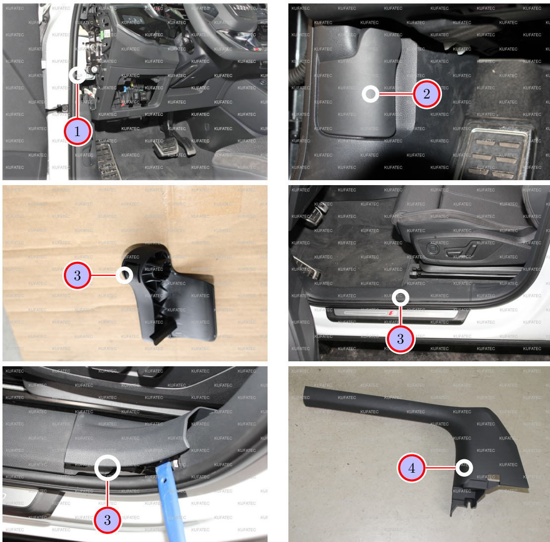
Figure 6: Disassembly A-column covering / sill trim driver's side
