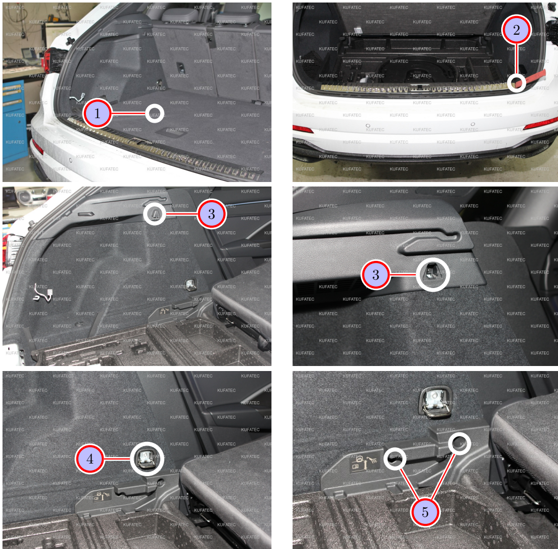
Figure 8: Disassembly trunk covering driver's side
