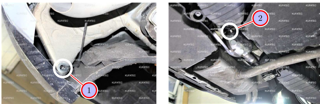
Figure 9: Cable routing to the sound generator
