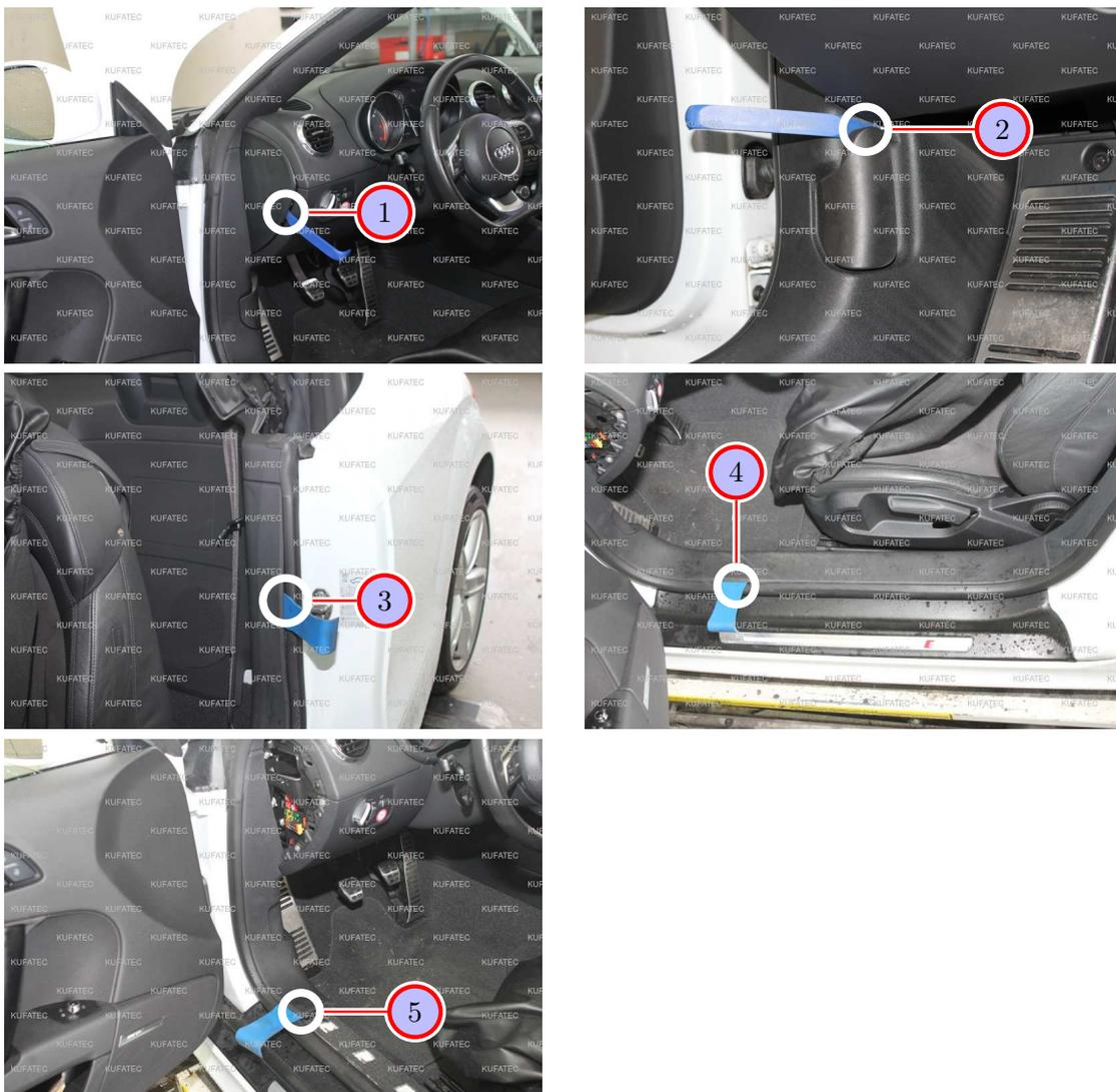
Figure 4: Removing trim panel driver's side
