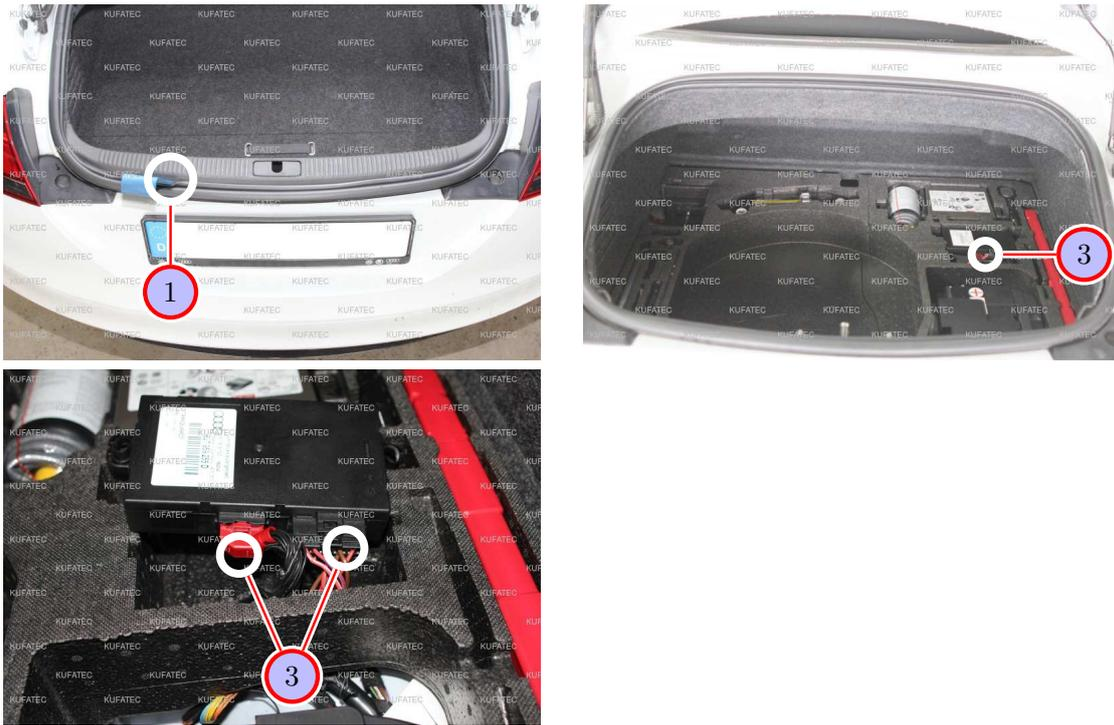
Figure 8: Removing cover parts trunk
