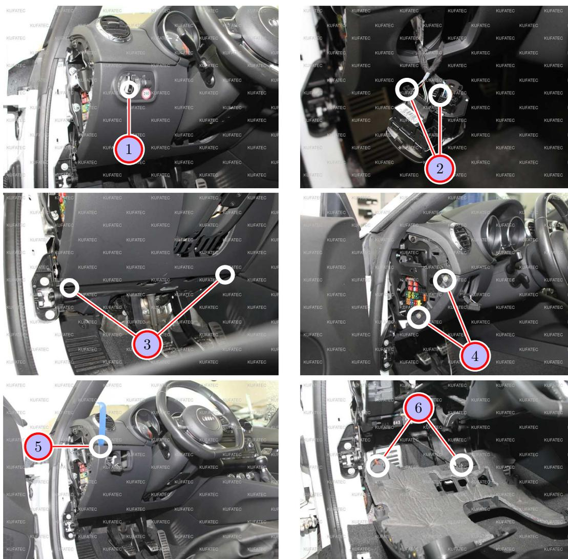
Figure 5: Removing lower trim panel of the dashboard
