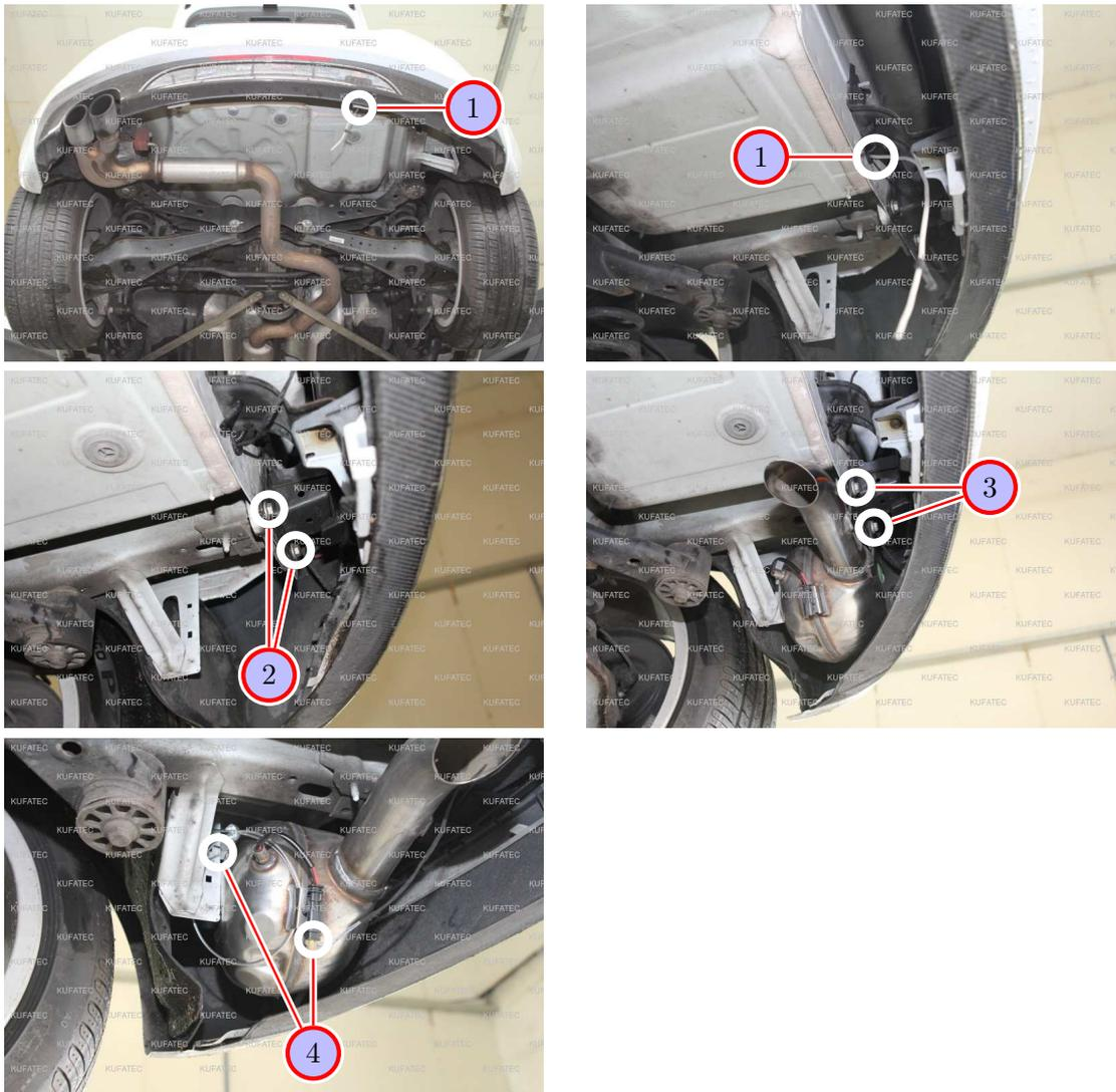
Figure 10: Installation sound generator
