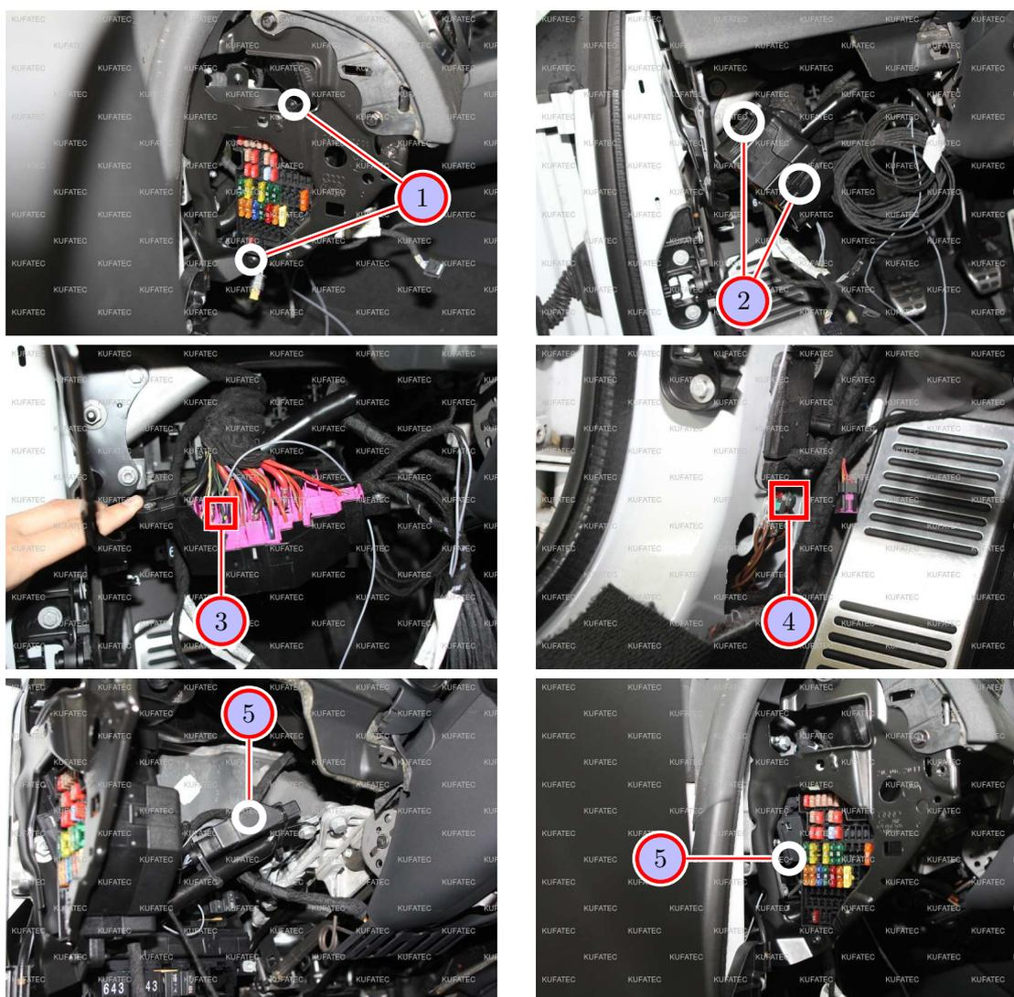
Figure 7: Connection ignition lead / ground
